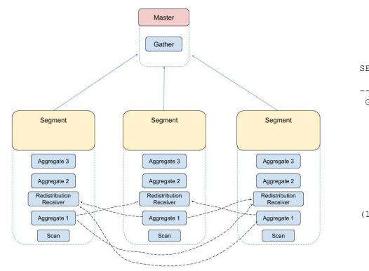
SELECT avg(distinct c3) from t1 group by c2; QUERY PLAN Gather Motion 3:1 -> HashAggregate Group Key: t1.c2 -> HashAggregate Group Key: t1.c2, t1.c3 -> Redistribute Motion 3:3 Hash Key: t1.c2 -> HashAggregate Group Key: t1.c2, t1.c3 -> Seq Scan on t1 (10 rows)
